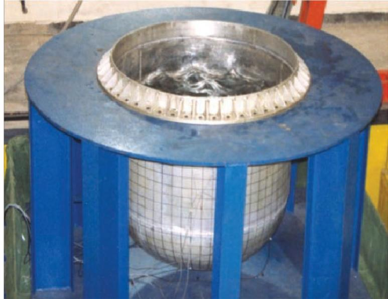
Shake table for seismic simulation
