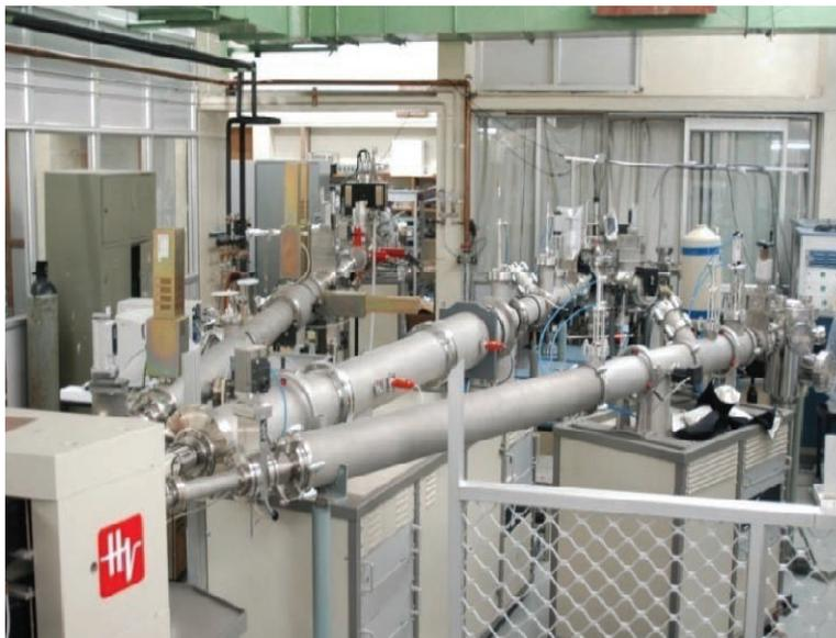
Beam lines and experimental stations built around a 1.7MeV tandem accelerator, used for Rutherford back scattering & channeling, and synthesis of nanostructures.
