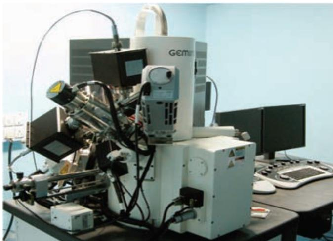
Field Emission Gas SEM-Focussed Ion Beam (FEGSEM-FIB): Cross Beam facility.
